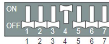
Figure 132: Heat Pump System DIP Switch Setting on Outdoor Units (Manually Set).
